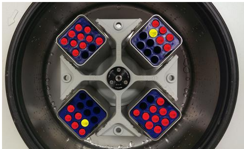
Example of a loaded centrifuge, where a yellow dot indicates a shorter volume tube
